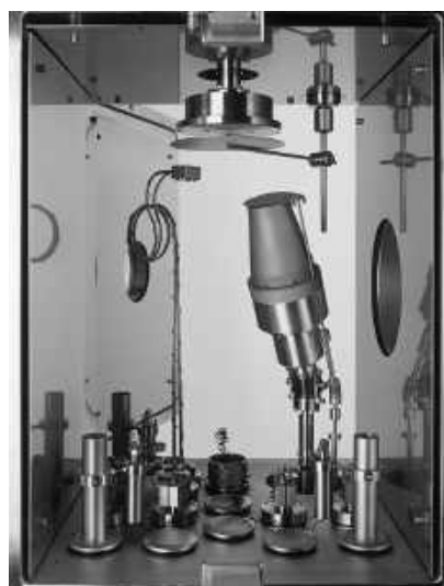
View through the vacuum chamber: front sliding door and rear swivelling door open
