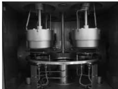
Chamber bottom: rotating substrate table with four heating stations Chamber top: four magnetron sputter sources
