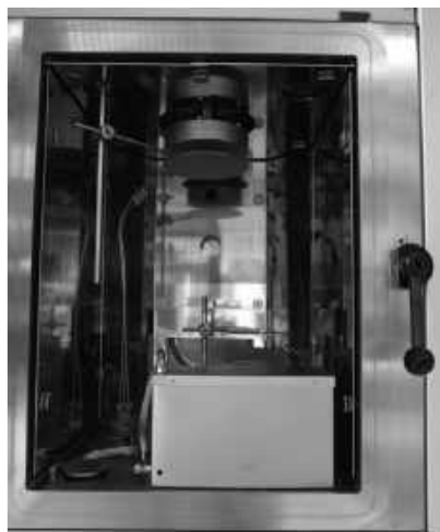
Rotating and water-cooled substrate table
