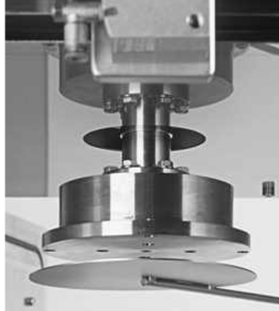
Rotatable and temperature controllable substrate holder with substrate shutter
