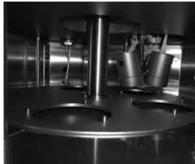
Coaxial hollow shaft drive for eccentric rotation and positioning of several substrates, with separate shutter table
