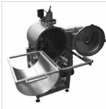
Opened coating chamber with retracted substrate receiver
