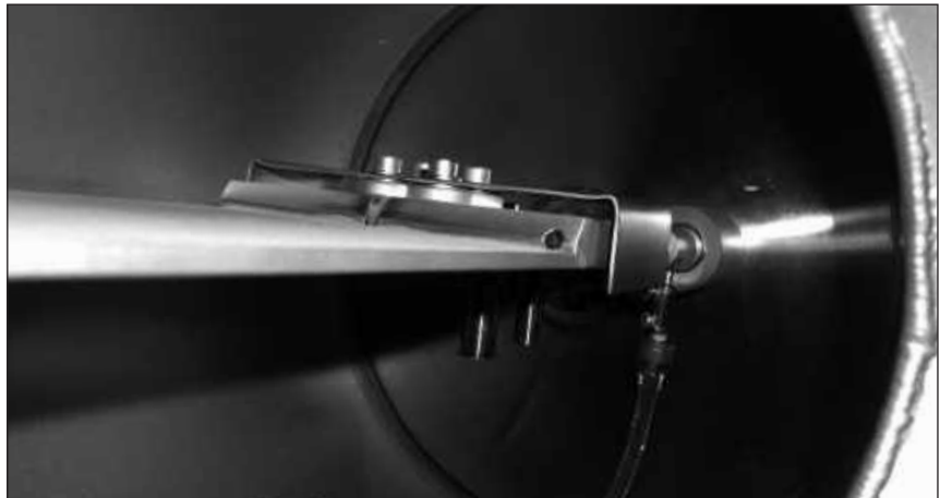
Insulated substrate fork with RF bias connection
