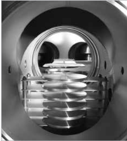
Design example: Automatically controlled substrate magazine with robot arm access
