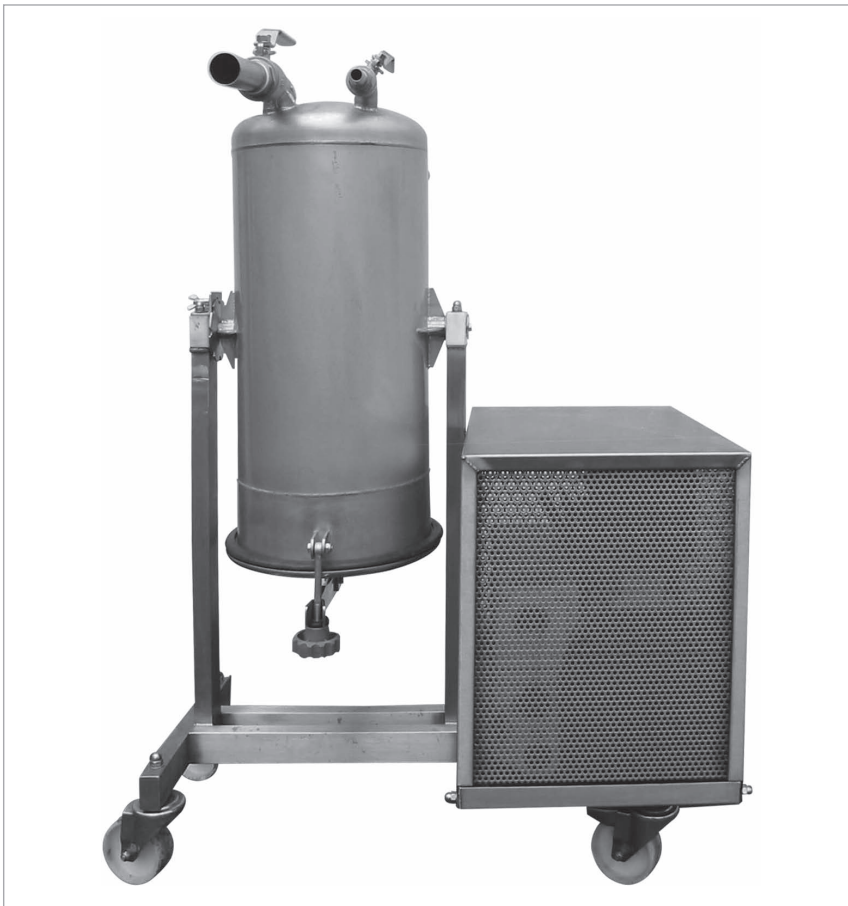
Spinal Cord Vacuum System for sheep and lamb equipped with SV65B HYDRO. With courtesy of TERMET, France.
