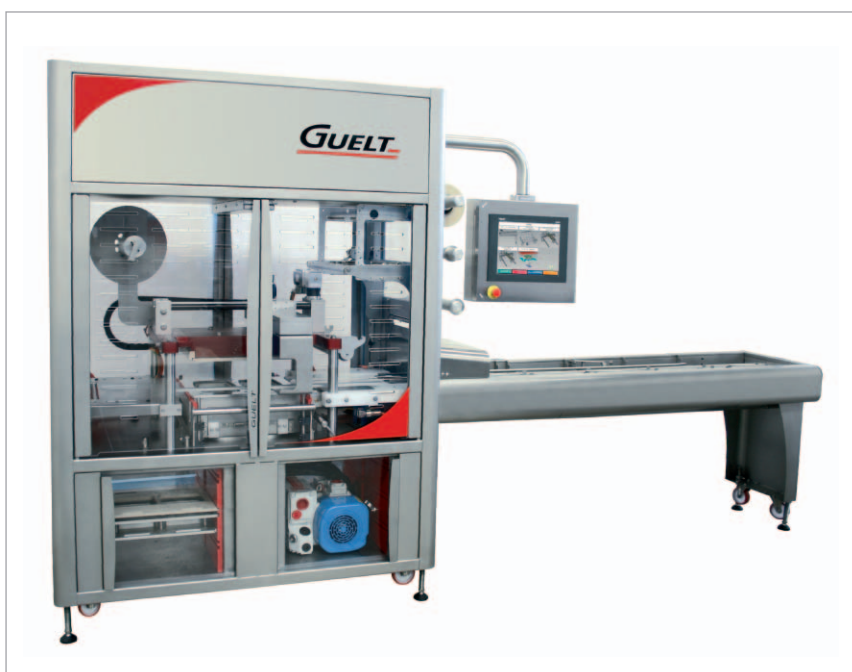
In-line tray sealer OPP2000, 100% electrical and connected. With courtesy of company GUELT, Quimperlé, France.
