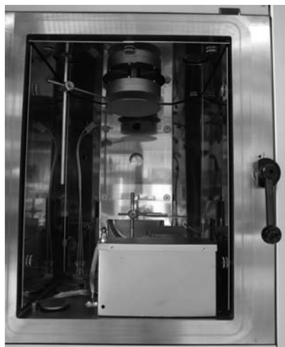
Rotating and water-cooled substrate table
